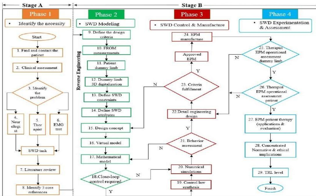
Figure 2: Flowchart of soft wearable devices methodology.
